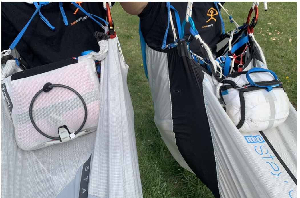
The rescue pod of the Stay Up 2 on the left is placed in a recess, and the one of the Stay Up 1 on the right is just laid on the pod, thus less stable.
