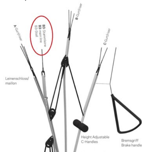
Nova Mentor 7 light : The B lines at the wing tips are attached on an additional strap between the A and B straps
