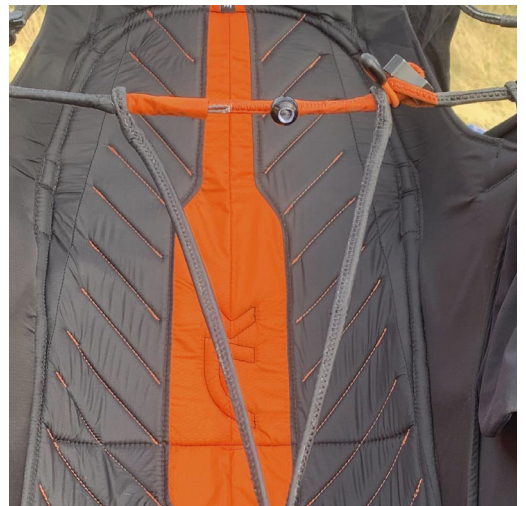
The front closure (Lyros Dyneema 4mm) is adjustable thanks to the black ball in the center.
