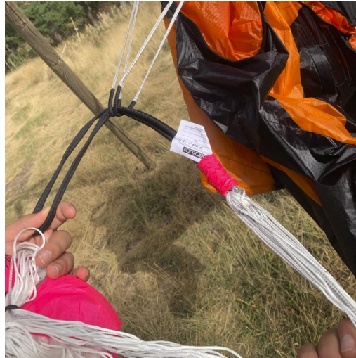
The reserve parachute is secured with a lark's foot knot, and the Y-bridle is attached behind the shoulders.
