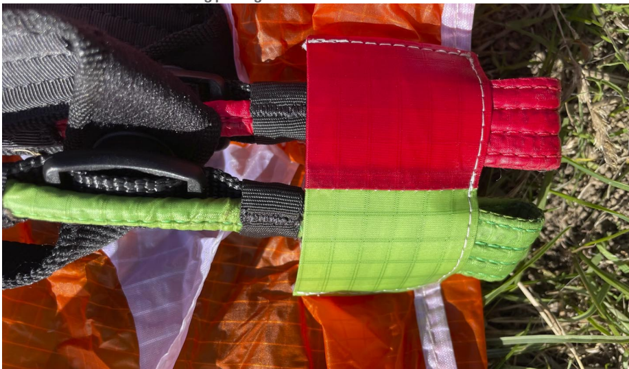
Practical details: Hooks to hold the leading edge in place on a steep slope, and fasteners for the risers during packing.
