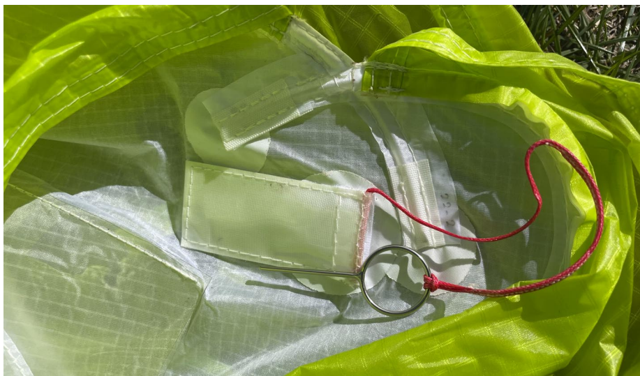
Practical details: Hooks to hold the leading edge in place on a steep slope, and fasteners for the risers during packing.
