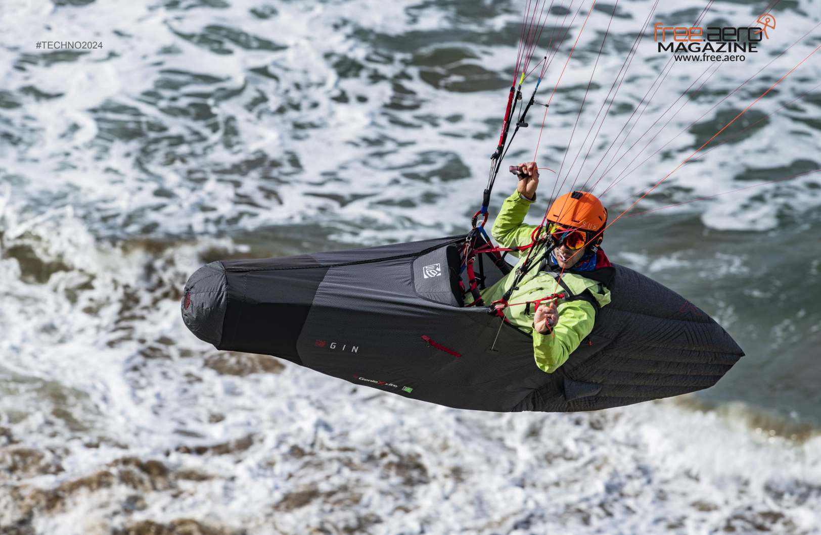
Good maintenance of the aerodynamic shape, and the tail remains well filled thanks to the air intake, which is sufficiently rigid.
