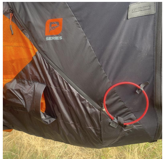
A Velcro strap keeps the reserve parachute deployment handle close to the harness.
