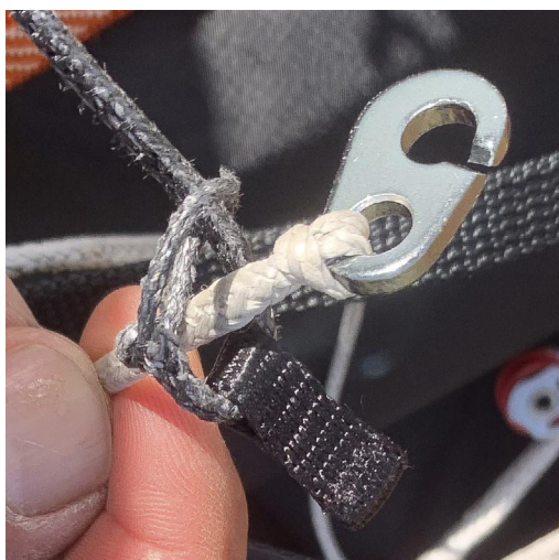
Attachment of the riser with a lark's foot knot.
