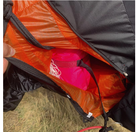
The location of the reserve parachute. Installation is easy and numbered in sequence.
