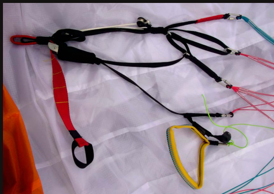
Thin risers have become standard on ITV wings
