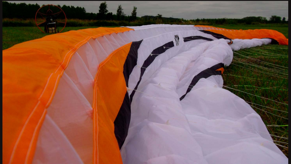
Rods at the leading edge, small air intakes, thin lines, no doubt about it, we are definitely looking at a latest generation wing.
