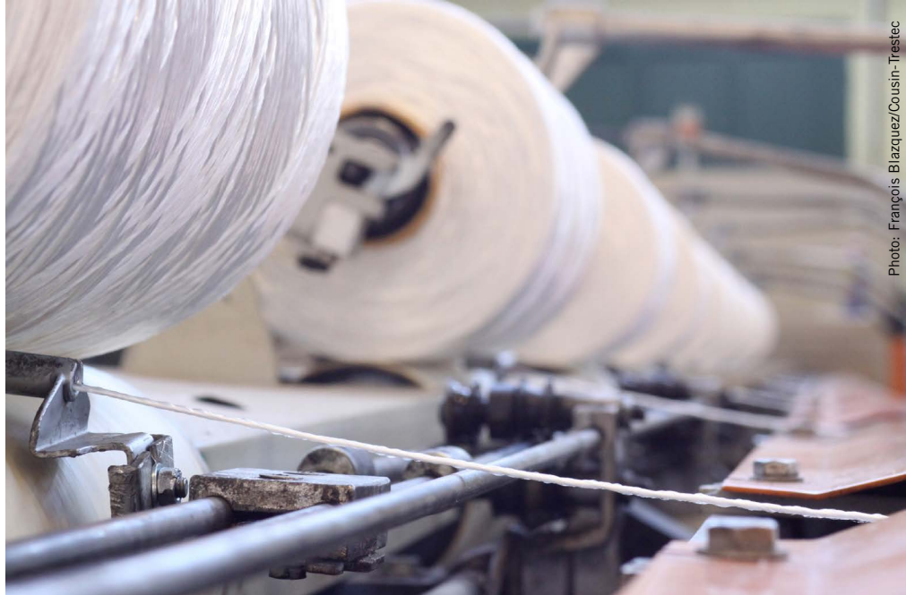
Dyneema cord being made at Cousin-Trestec. This manufacturer uses Dyneema fibre from the Dutch company DSM, owner of the Dyneema name. The threads are woven and coated according to requirements.
