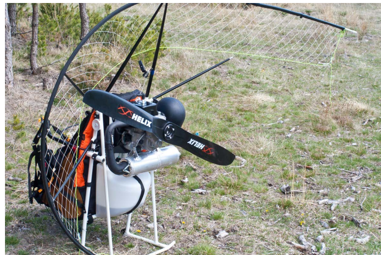
Lightweight chassis, motors that get lighter and lighter. Above, the famous EOS 100 on a Miniplane chassis. Below, a Miniplane chassis being put together: The cage made of glass fibre is put together like a tent with hoops.
