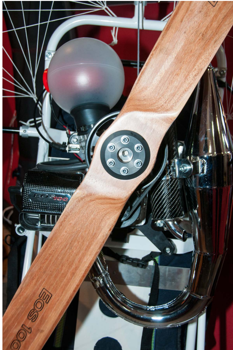
Lightweight chassis, motors that get lighter and lighter. Above, the famous EOS 100 on a Miniplane chassis. Below, a Miniplane chassis being put together: The cage made of glass fibre is put together like a tent with hoops.
