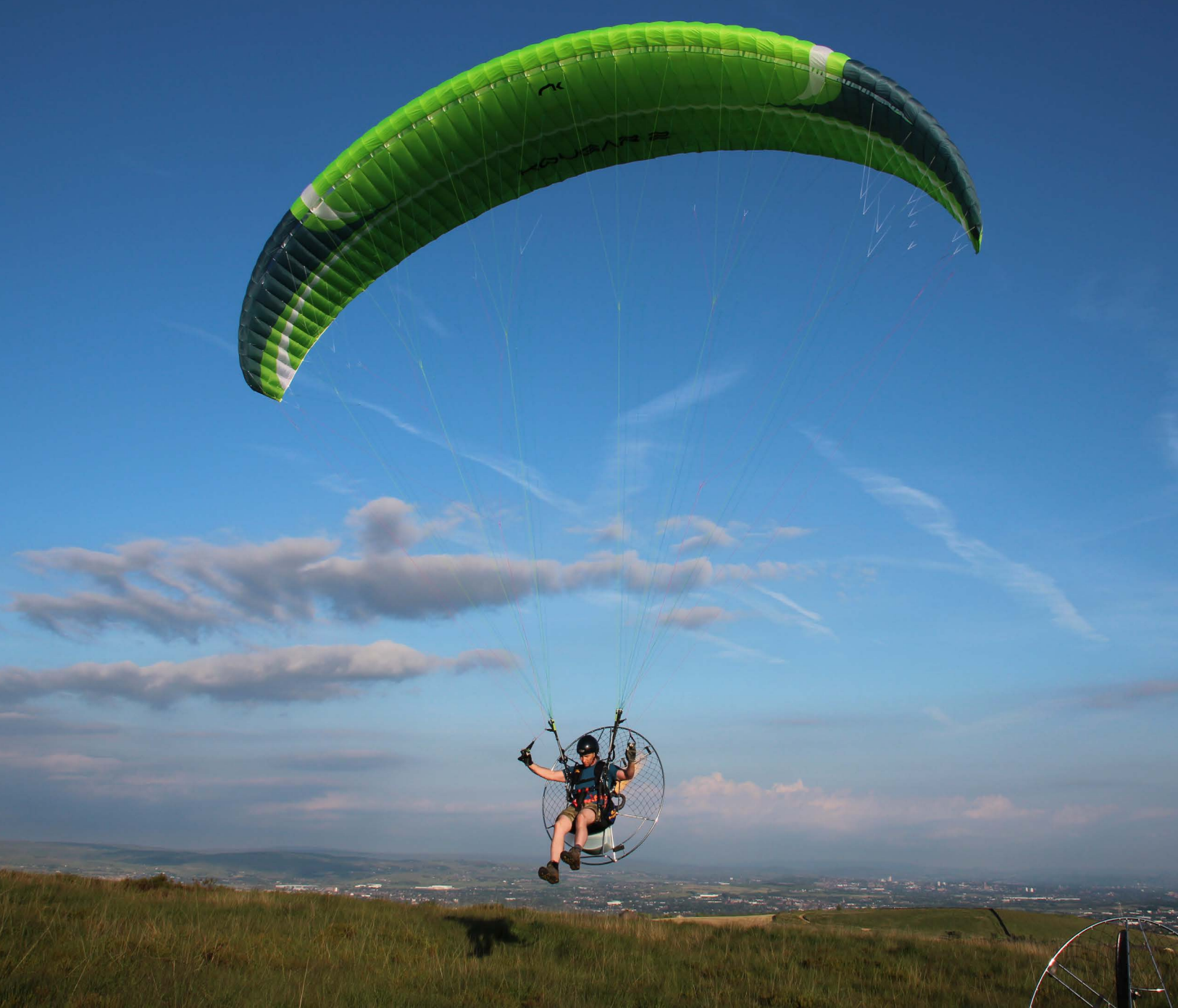
As in the picture of this Niviuk Kougar 2 reflex wing, the SharkNose is being added to more and more intermediate wings, both paraglider and paramotor.
