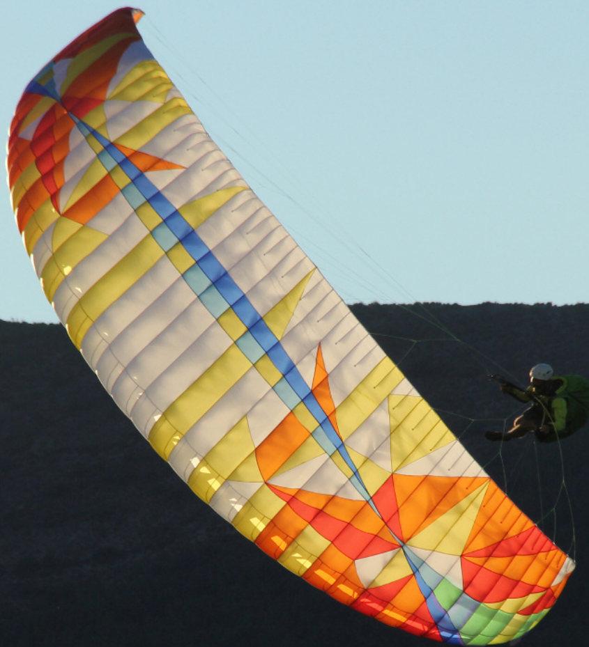
The "Low-EN B" Echo, the lightweight version of the Epic, with a pronounced SharkNose, mini-ribs, CCB (3D-Shaping), and a unique design...
