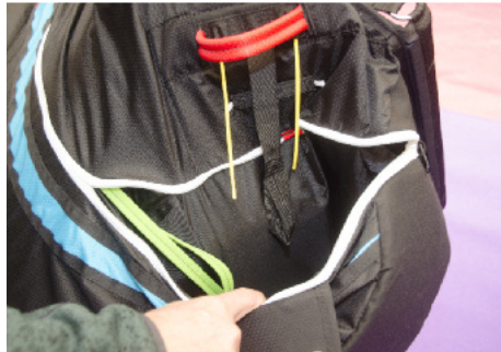
Reserve containers which close with a zip and have a strap linking the handle to the pod.
