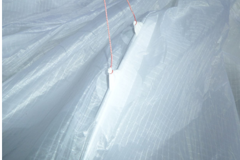
Checking the leading edge, the 3D Shaping reveals a constrained short rod which gives the SharkNose its shape. A double row of As, very close together supports the SharkNose.
