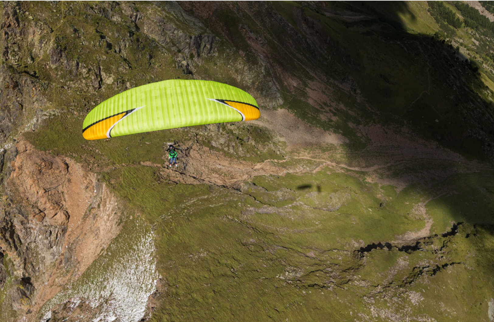
Clearly visible: the 3D Shaping in both the leading and trailing edge.
