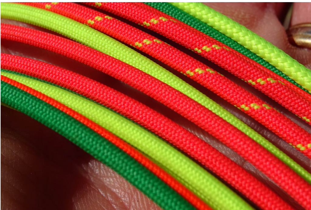
Lower lines: Edelrid Technora 7343: 420/340/280/230. Higher up there is also Edelrid Dyneema.
