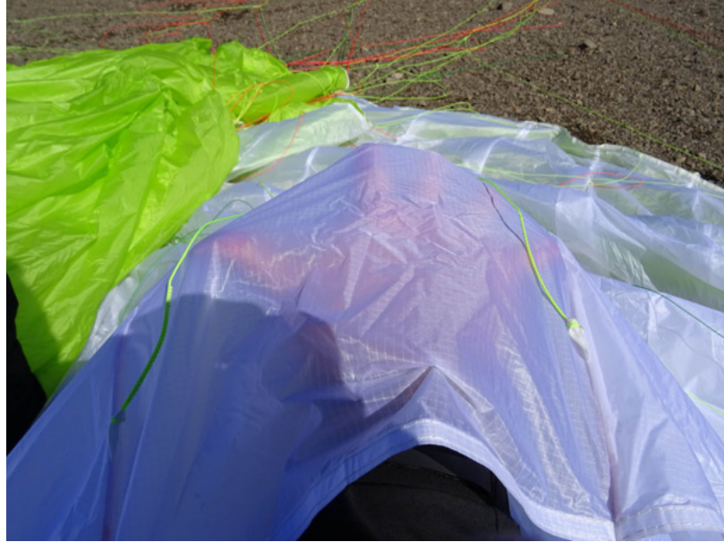
The lower surface: Dominico 20D soft finish.
