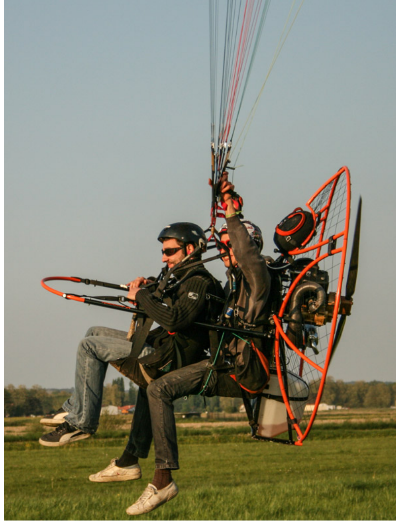
The roll bar serves above all at take-off: it aligns the passenger and separates him from the pilot and, above all, from the blade... Shown here, Kangook's old roll bar.
