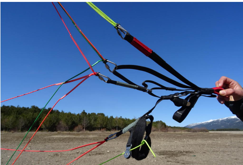
A relatively classic tandem riser with trimmers.
