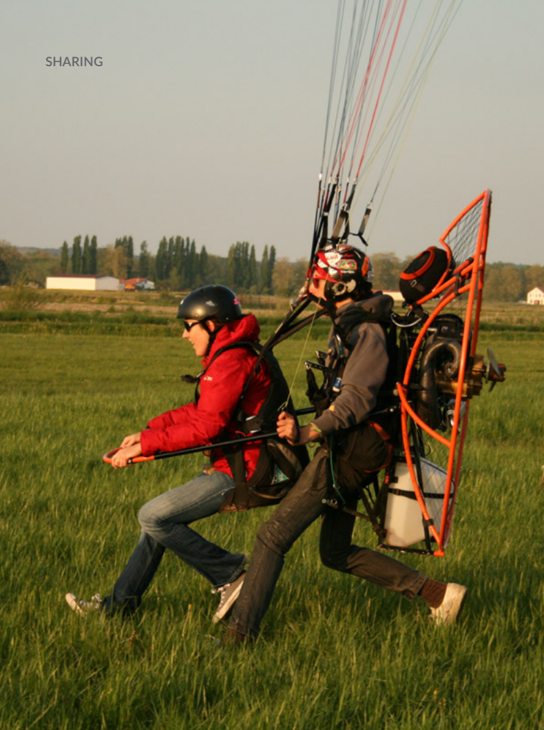
The roll bar serves above all at take-off: it aligns the passenger and separates him from the pilot and, above all, from the blade... Shown here, Kangook's old roll bar.
