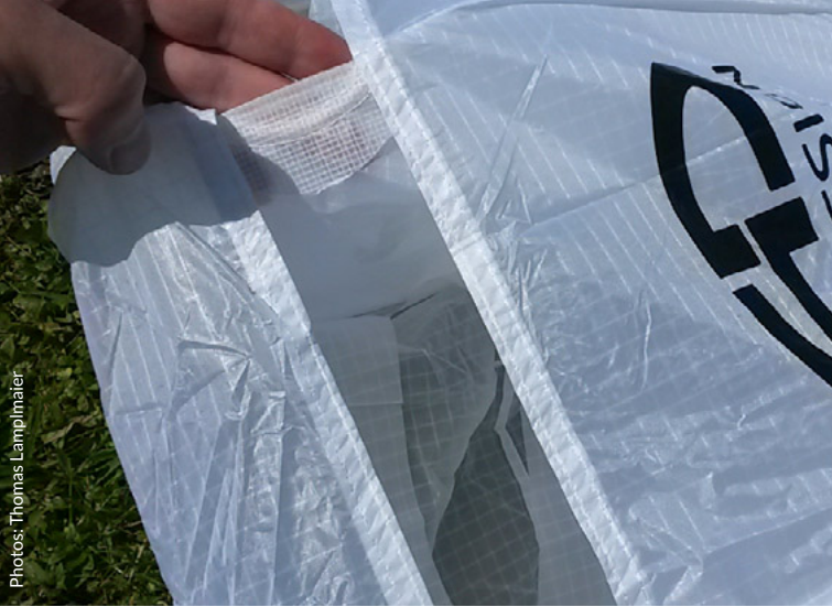
Checking the leading edge, the 3D Shaping reveals a constrained short rod which gives the SharkNose its shape. A double row of As, very close together supports the SharkNose.
