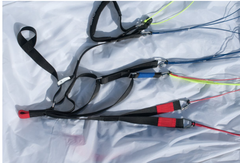
The relatively thick and very solid risers contribute to the final weight.
