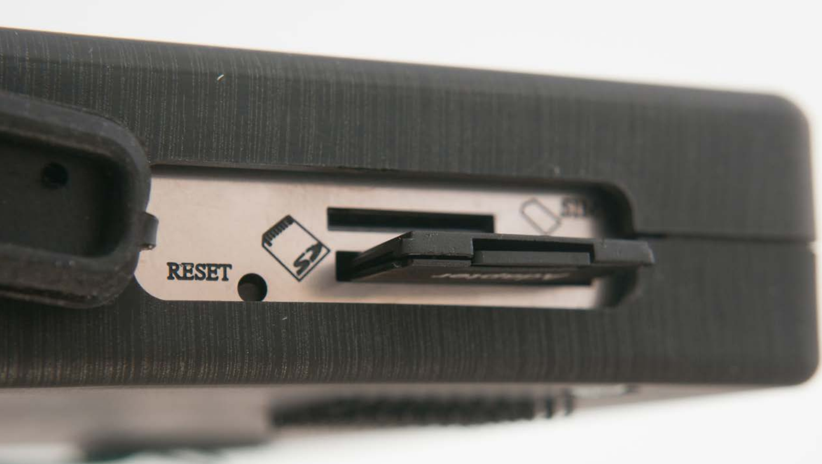
Above the slot for the SD card is the slot for the SIM card which is useful for live tracking.
