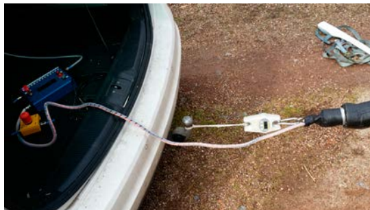
The cable is fixed to the tow bar of the car (here with a spring balance to test it).
