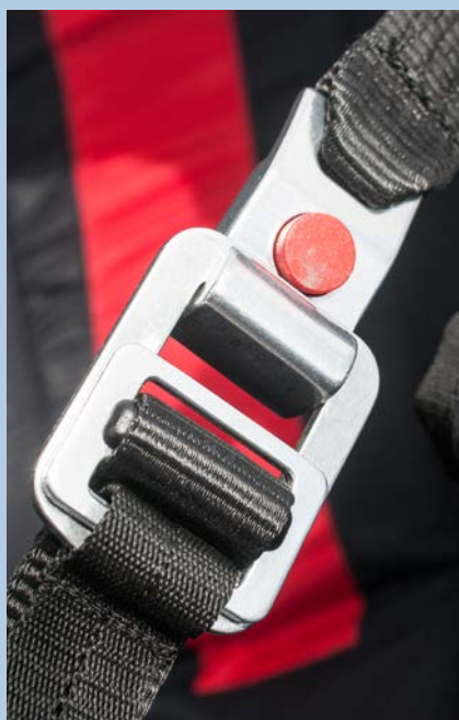
This type of buckle, also made by Finsterwalder and used by several makes, can't open under tension. On the other hand, if the button releases, the buckle could open when the strap is not taut. A safety notice was issued concerning the rare cases where the button could come out of its housing.
