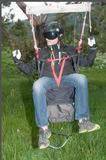
A harness with a Get-Up system. This harness isn't affected by the problem because its flat buckle fastenings can't open all by themselves.
