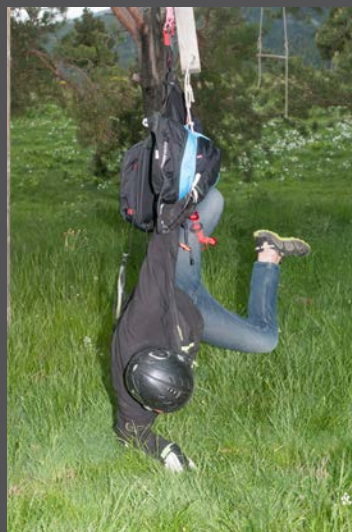
The pilot is suspended by only a single strap, and one that is loosely done up, in the case of a Get-Up system.
