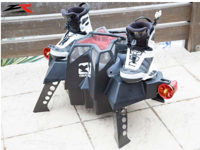
Four jet engines in the middle to give the lift and two other motors to control it on either side.
