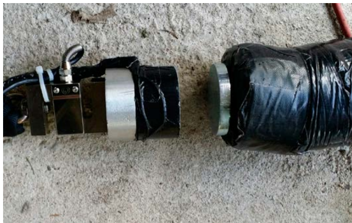
An electromagnet which is cut in case of overload.
