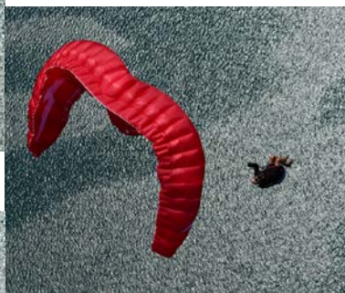
Manufacturer's photos: A 'frontal' sequence on a Swing prototype equipped with a RAST system. The reinflation is progressive; it's actually an advantage which was confirmed during our tests.
