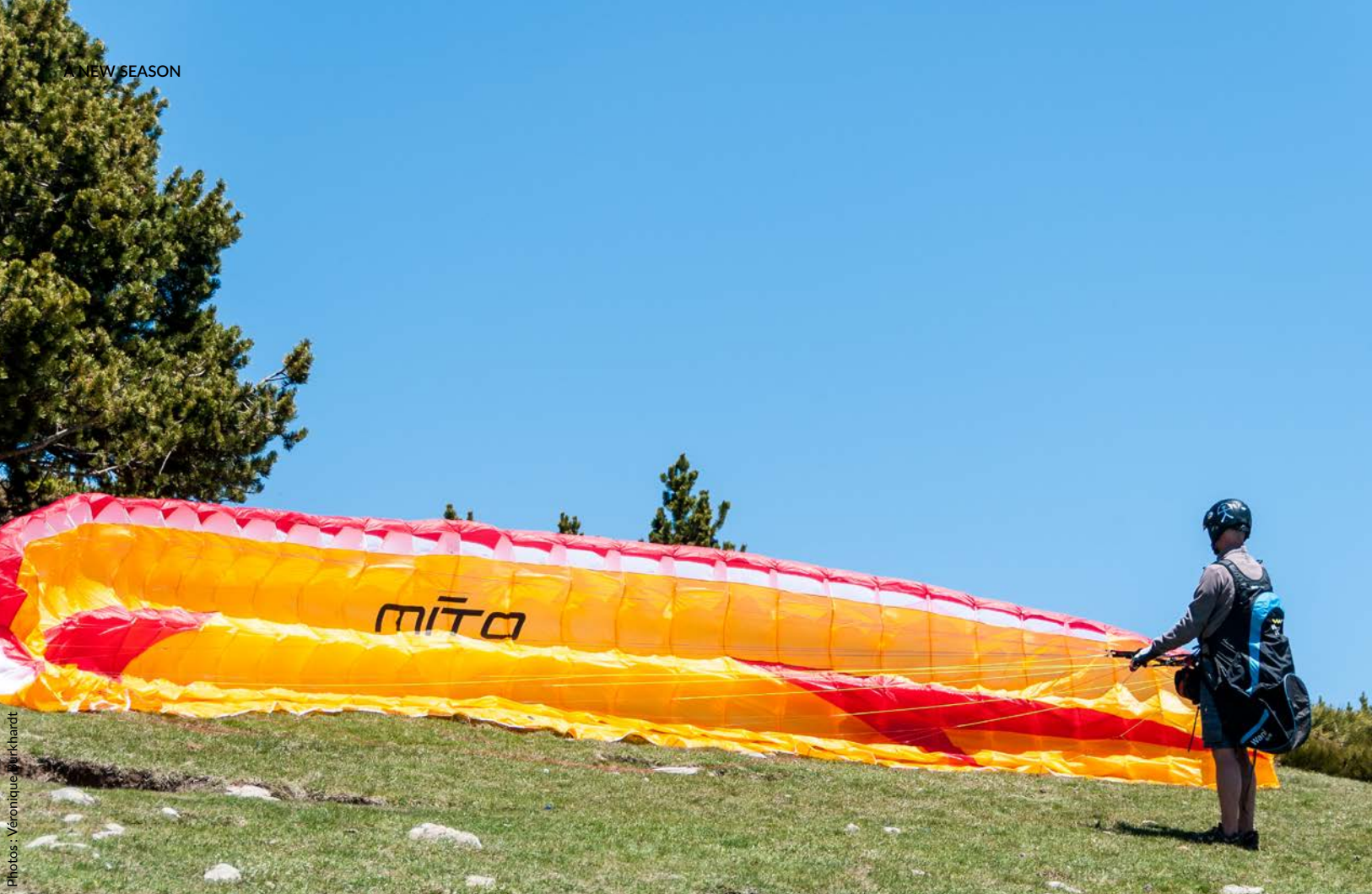
The RAST system rib is visible on this photo in the front third of the wing. You can also see the use of mini-ribs on this EN A.
