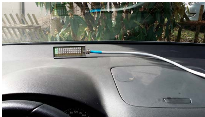
The driver can check the tension thanks to the coloured LED lights. All he has to do is regulate his speed so that they stay green.
