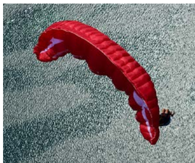
Manufacturer's photos: A 'frontal' sequence on a Swing prototype equipped with a RAST system. The reinflation is progressive; it's actually an advantage which was confirmed during our tests.
