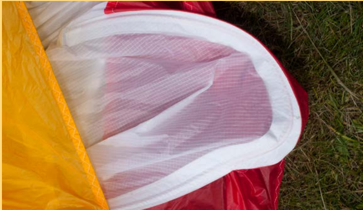
The rods form a light SharkNose
