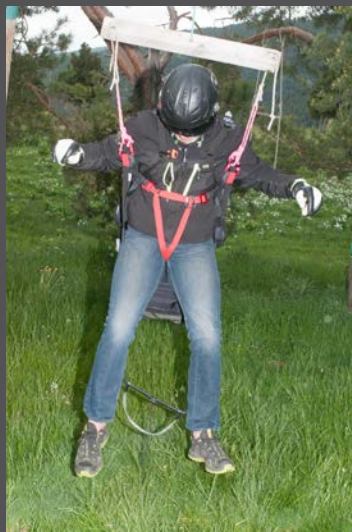
Even when loaded, as long as the two buckles are fastened, the pilot is obviously held securely in place.
