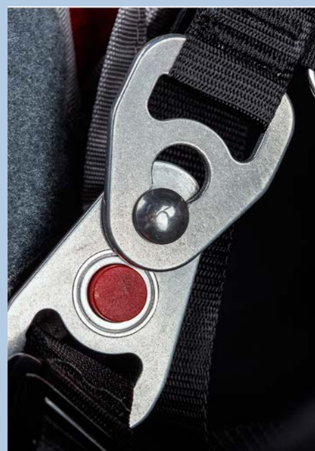
This type of buckle, also made by Finsterwalder and used by several makes, can't open under tension. On the other hand, if the button releases, the buckle could open when the strap is not taut. A safety notice was issued concerning the rare cases where the button could come out of its housing.
