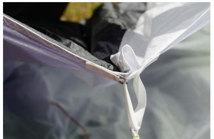
A classic way of increasing the manoeuvrability: using the controls shortens the trailing edge on the brake side.
