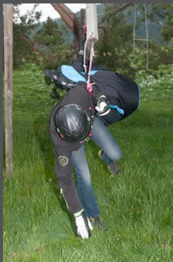
In particular, during a violent manoeuvre, the pilots arms can easily slide out of the harness.
