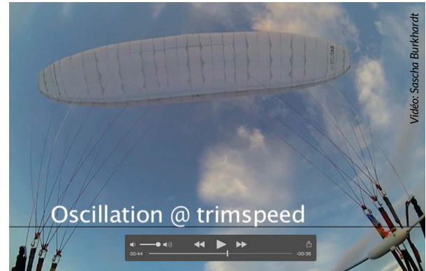
A short video showing the oscillations with hands up on the Batlite from Adrenaline (00:44 onwards) www.free.aero/videos/batlite_ppg
