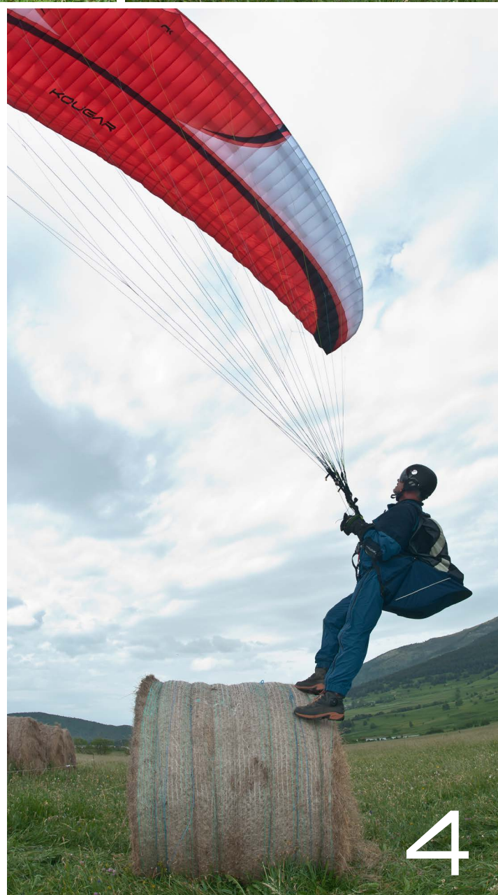
On the other hand, when the wind is weak, the brakes give more lift for climbing... Photos: Véronique Burkhardt
