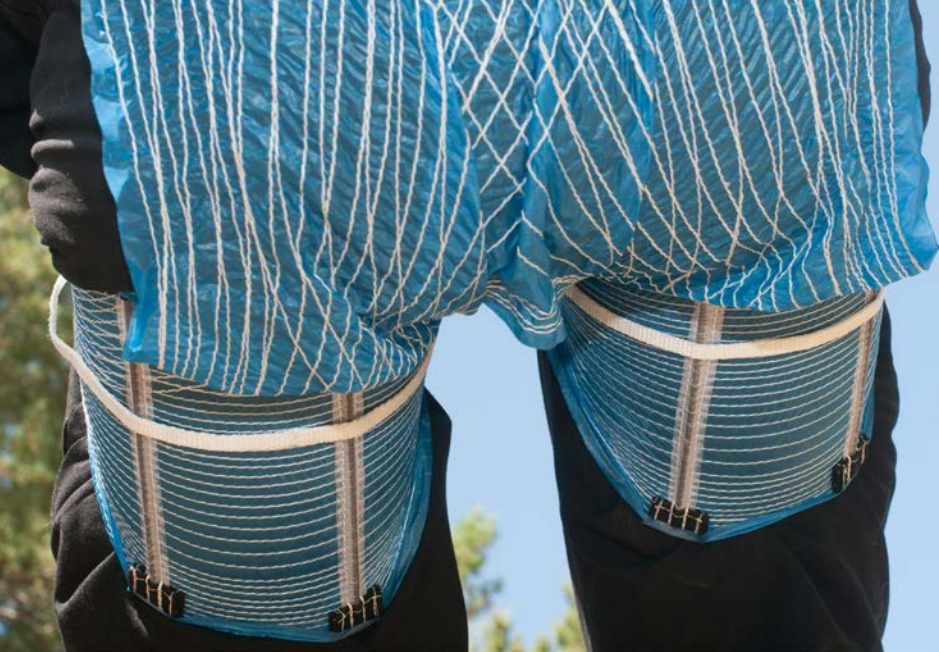
The carbon rods under the thighs work primarily in compression.
