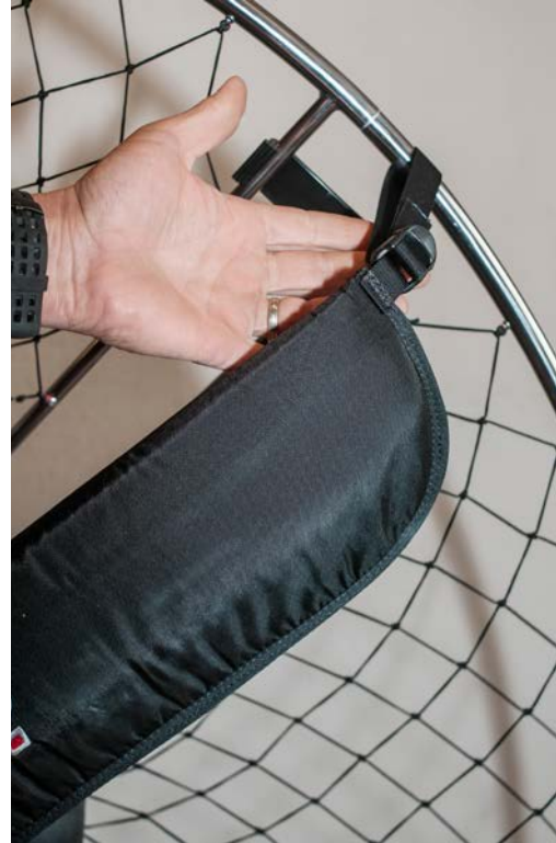
At take off, to warm the engine up, the blade can be blocked using this device. Obviously, remain on tickover so that the clutch doesn't engage, making the motor stall.
