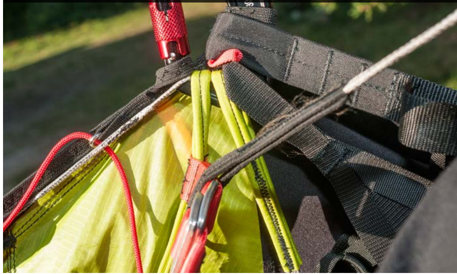
Lots of stitching judiciously placed, together with the straps, creates a complex system which guarantees that this 'bag of washing' takes on the correct shape. The seat of the Rangeair allows it to be flown in a sitting up position as well, if the pilot wants: an important advantage in certain situations requiring good downwards visibility, for example when landing out.
