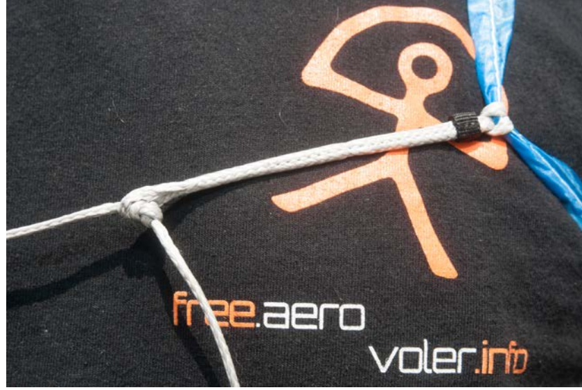
A buckle made up of a knot jammed in a loop which holds the shoulder straps in position.
