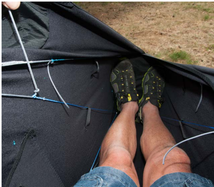
Middle: Perfect adjustment of the detachable pod is paramount. It is done with knots that the pilot moves just once along these lines. During our test, the latter got damaged during the handling necessary to adjust them. Since then, Advance have made some modifications.
