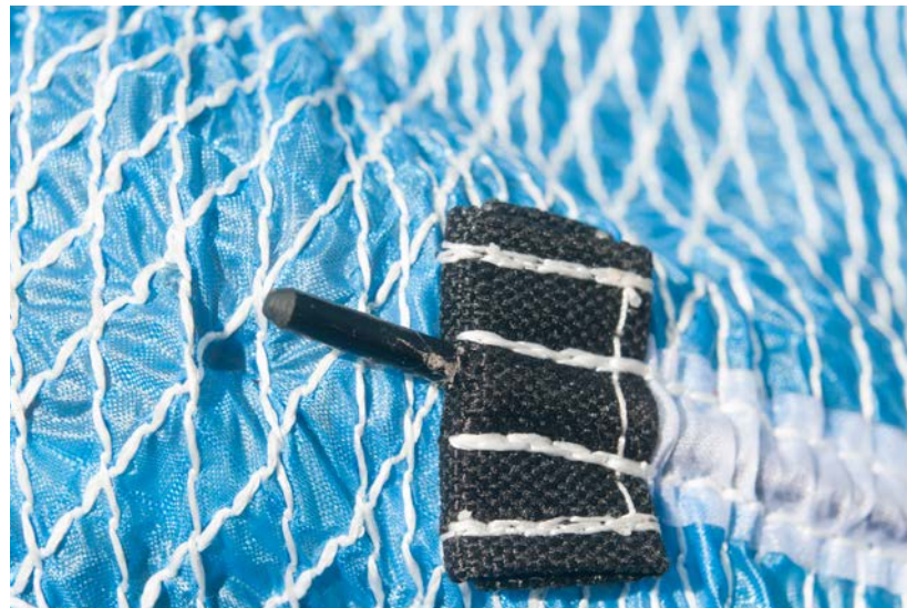
A small fault on the prototype we tried: a rod pierced the end of the strap covering it.
