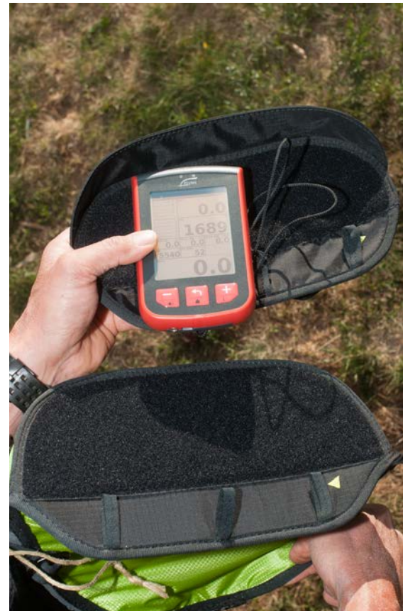
The instrument panel is removable and is attached by Velcro onto the ventral storage bag.
