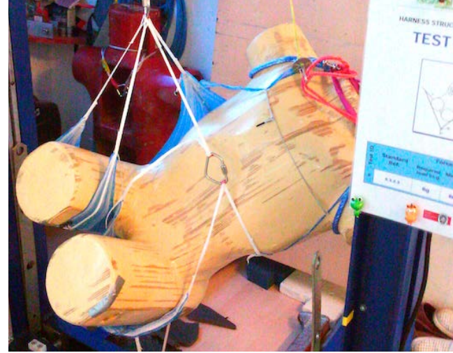
The F*Lite during the load test which allowed the concept to be validated. It survived 15 G which is equivalent to 1500 kg(!), and not a single fibre broke according to Ozone!
