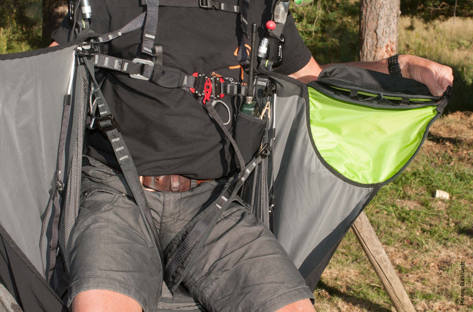
A buckle system with two buckles at the thighs and an anti-forget T for the waist. Worth noting, the radio pocket which has been included, a popular little detail.
