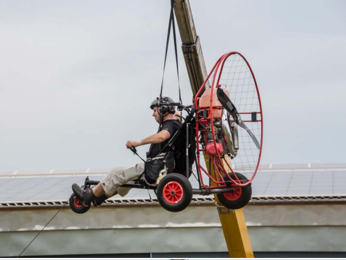
A good initiative at Ballenstedt: reserve throwing. There was more than one which wouldn't open, like the one on the right due to a mounting error.
