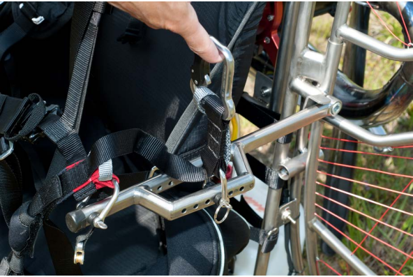
On these bars from FTR, you can clearly see the different holes allowing the hang point to be adapted to the pilot's weight. The heavier he is, the further forward the attachment of the risers will be on the bar.
