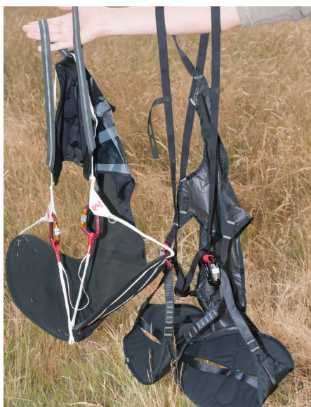
The String from Neo (left) weighs 300 g. The Everest 2 from Supair (right) weighs 450 g. Photo: voler.info
