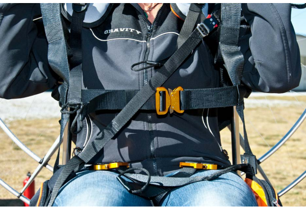
On this Nirvana trike, it's the diagonal strap which serves to compensate for the torque of the motor.
