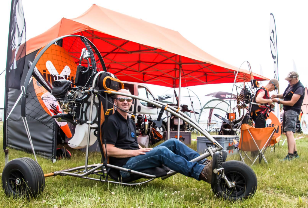
The German make Simplify has had rapid success in Germany and Austria with its 'light and easy' concept. The foot launch machine with EOS 100 only weighs 17.5 kg. The trikes in titanium exist in several versions between 22 and 45 kg. www.simplify-ppg.com
