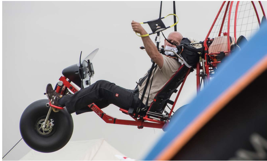
A good initiative at Ballenstedt: reserve throwing. There was more than one which wouldn't open, like the one on the right due to a mounting error.
