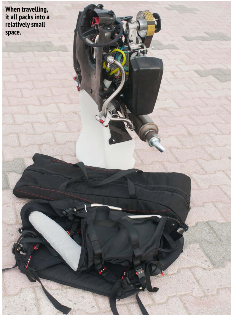
Like all the Adventure chassis, the engine is very compact on the pilot's back and leaves him lots of freedom. In addition it weighs 30% less than the numerous other engines with the same power.
