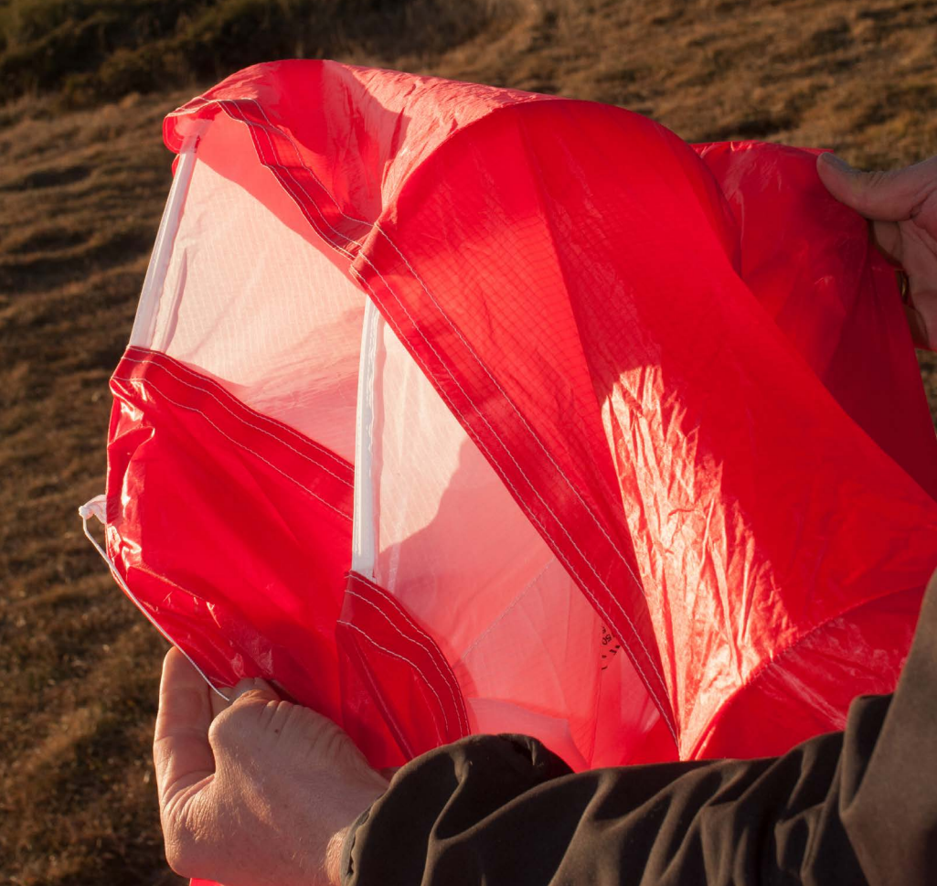
Leading edge rods in the large openings: inflation is very easy, the load take up progressive.
