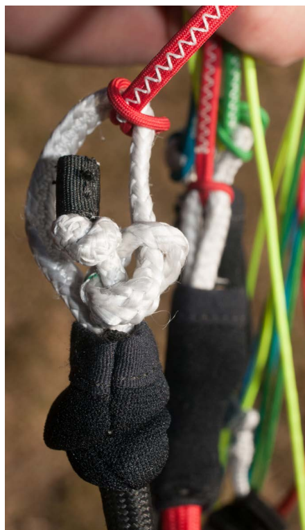
The softlinks on the Sitta are different: they comprise a lark's head knot blocking against a stop knot.
