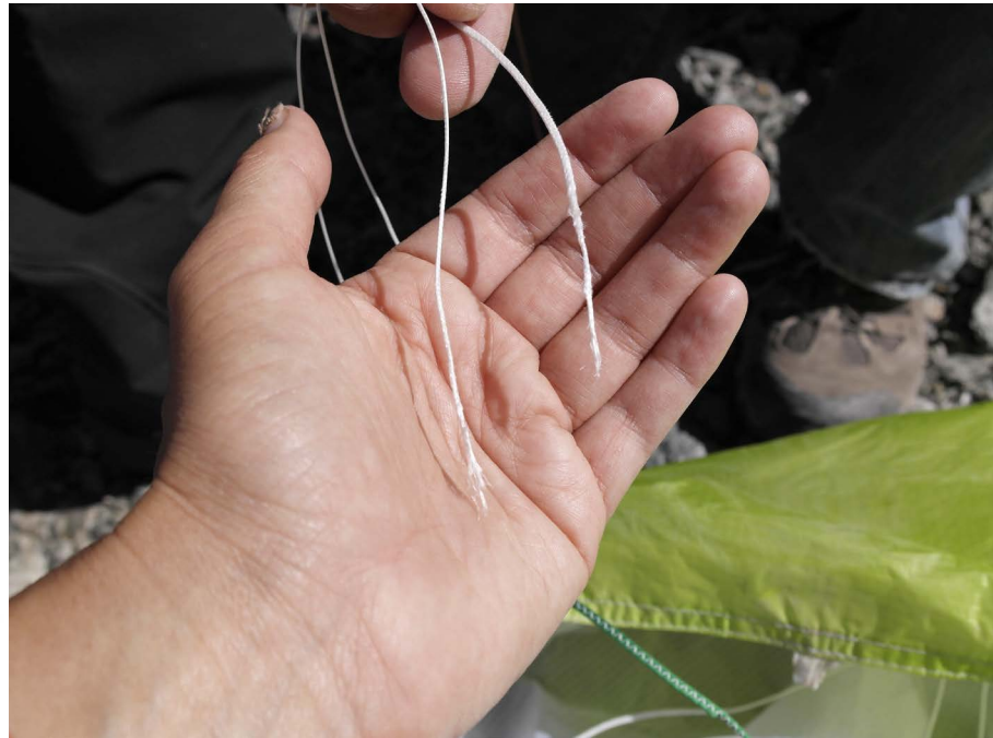
Breakage of non sheathed lines: this can happen, but it isn't the main problem with them. www.profly.org
