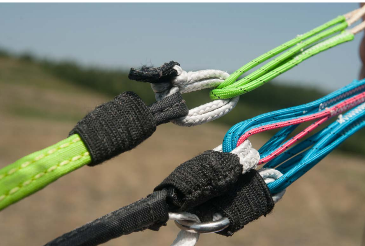
On the Plume, the lines and the risers are joined by Niviuk's 'LI-NK' softlinks.
