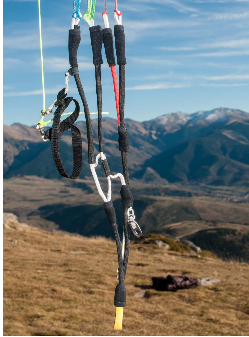
The weight has been reduced though the choice of fabric and by using Dyneema risers.
