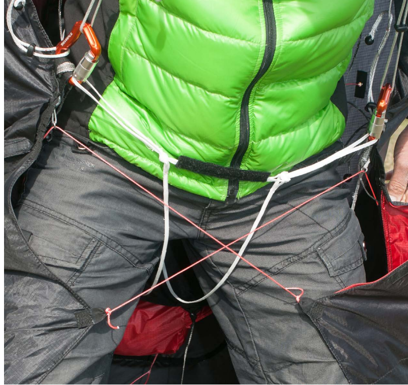
Skywalk Range X-Alps: Dyneema chords instead of straps
