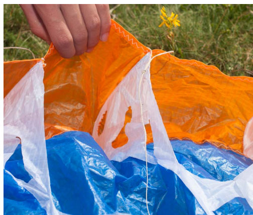
The detail on the Skin Plume: a major part of its excellent profile is no doubt the work of the Nitinol leading edge rods.
