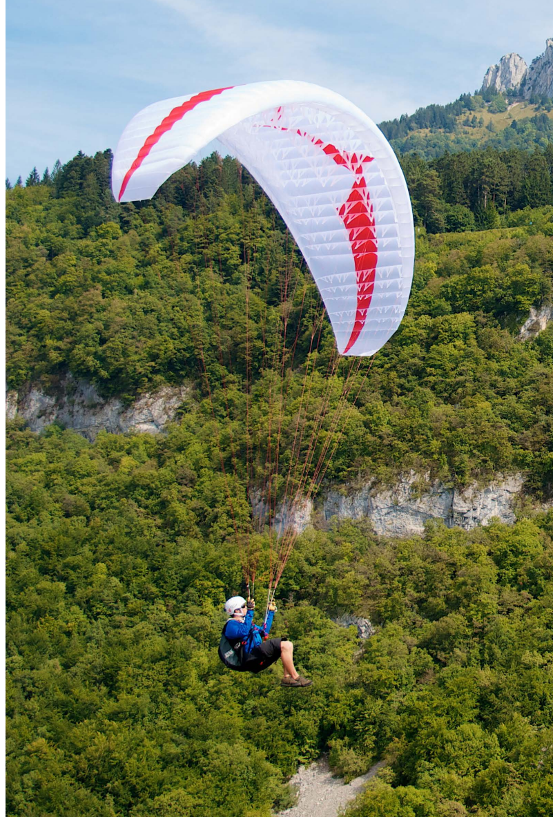
The XXLite from Ozone (2012): still the first generation of single skins, but with relatively good performance compared to the Batlite. On the other hand, as far as handling is concerned, the XXLite is one of the most demanding single skins. Photo: Loren Cox/Ozone
