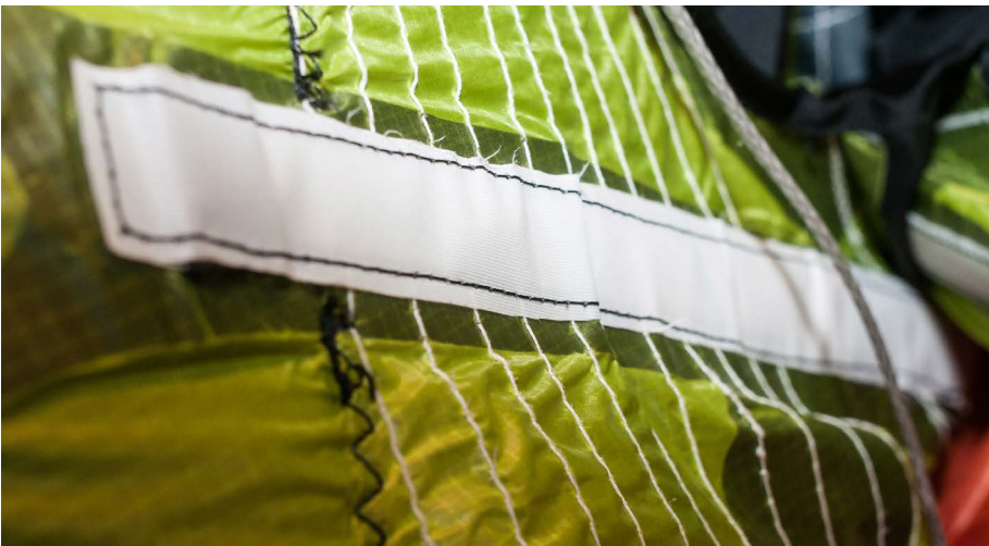
The glass fibre slats for the compression forces.
