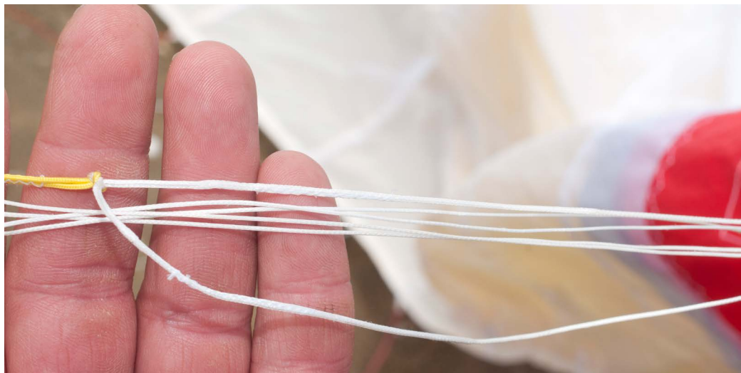
For unsheathed lines, the manufacturers use Dyneema (above), Aramid (below) and Vectran. Dyneema is often white whilst the others are brown, but the colour doesn't always tell us the difference. Dyneema is dimensionally less stable than the other fibres.
