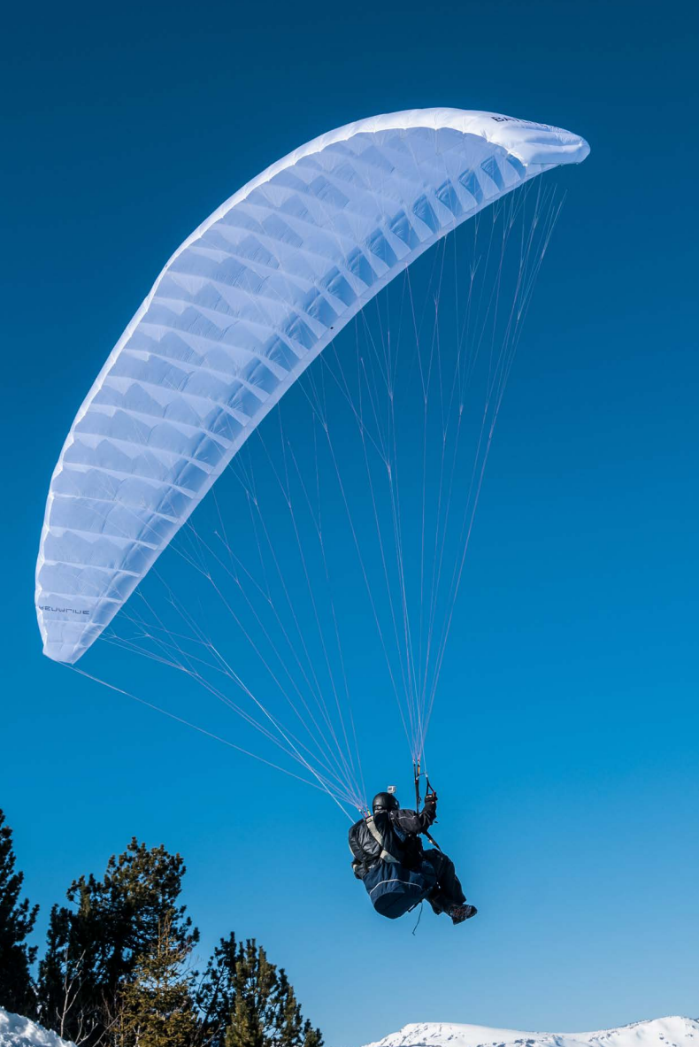
The Batlite from Adrenaline, based on the Barretina plans, shown here when we tested it at the beginning of 2013. The Batlite is the most lenient wing, as far as handling is concerned, out of all the single skin wings. Photo: Véronique Burkhardt
