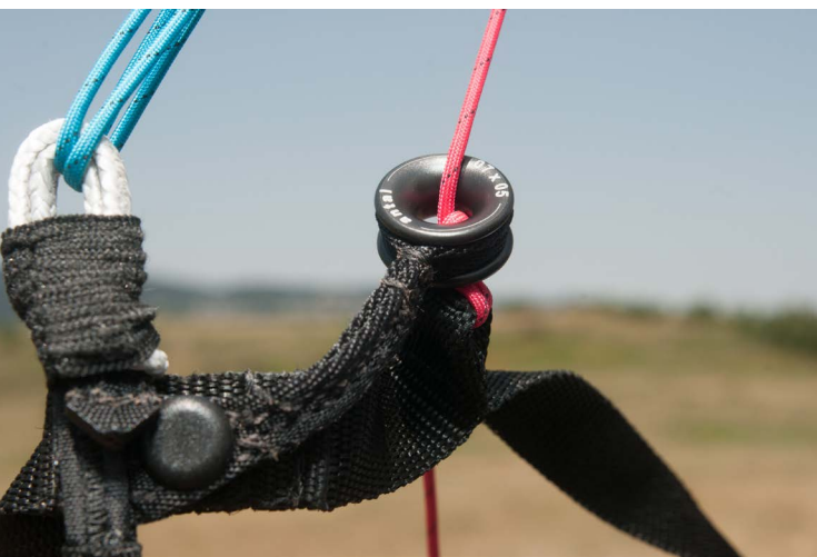
Obviously, a friction ring replaces the brake pulley on this ultra-light wing.
