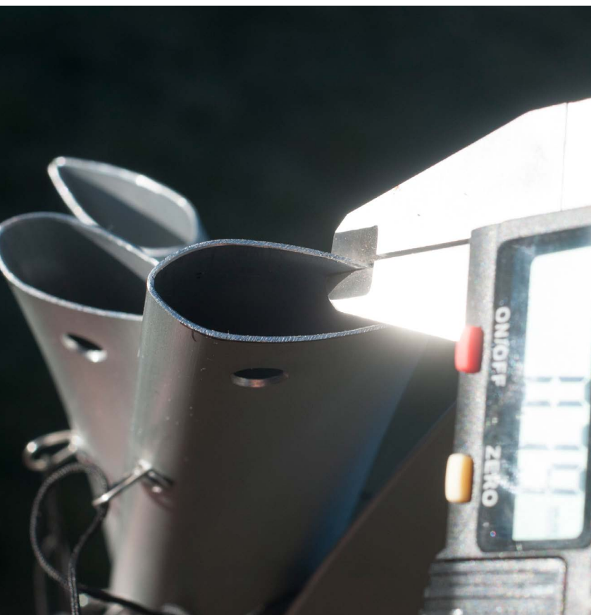
The hoops are very robust thanks to their profile, despite being so thin and light.
