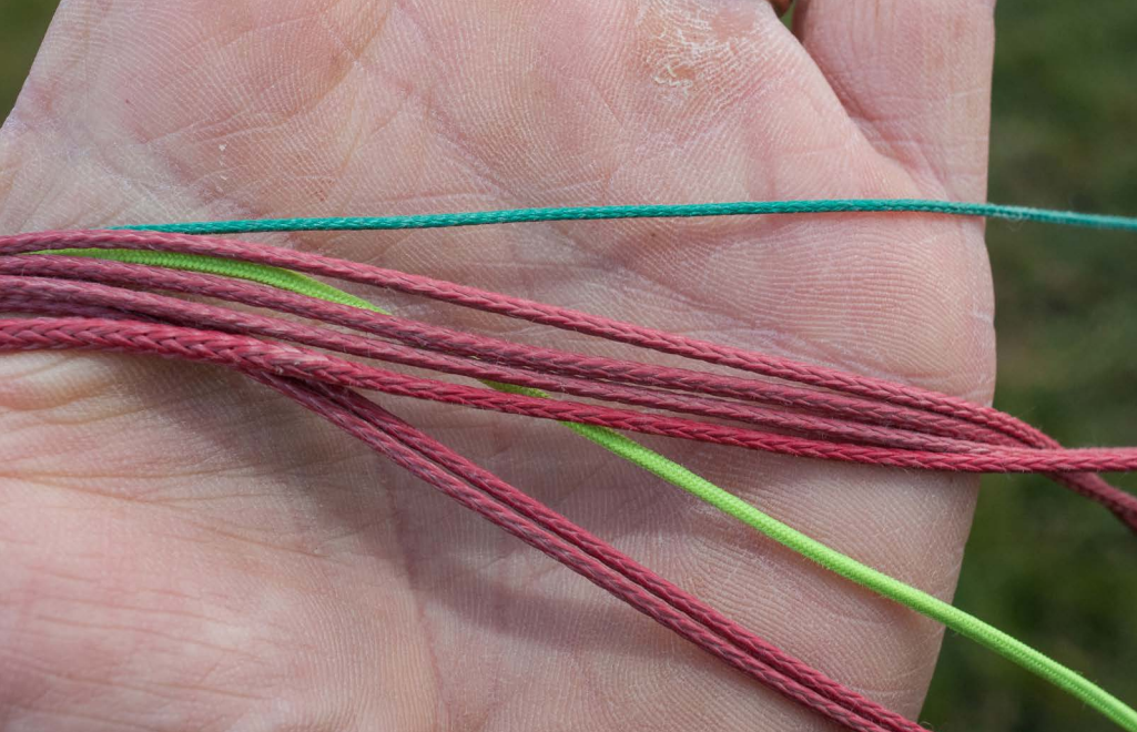
The unsheathed lines on the Air Design UFO 16, are mainly made from Edelrid Aramid.
