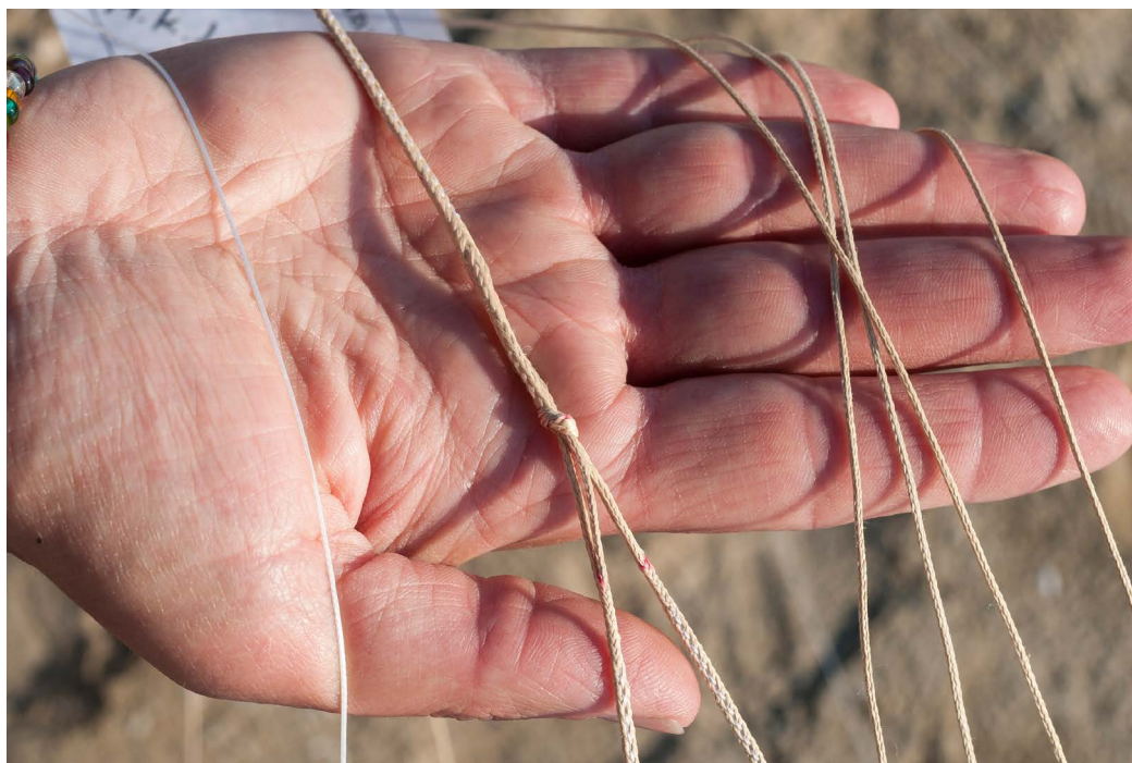
For unsheathed lines, the manufacturers use Dyneema (above), Aramid (below) and Vectran. Dyneema is often white whilst the others are brown, but the colour doesn't always tell us the difference. Dyneema is dimensionally less stable than the other fibres.
