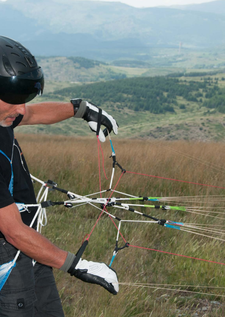
The plaited risers of the Skin Plume can be clearly seen.
