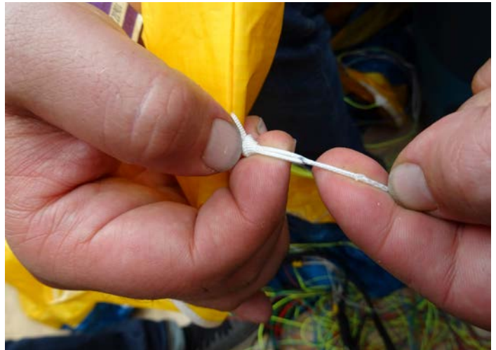
Inside the splice which forms the buckle on this thin line there is an extra line to make it stronger.
