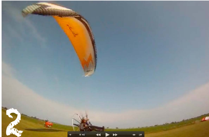
A collapse in the lee of the pylon.
