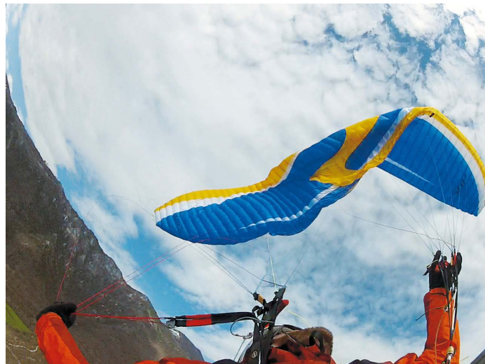
The same wing in a 'big' collapse. Here the DHV pilot managed very well without folding lines – but is it feasible for all modern wings?
