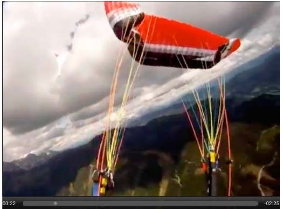
A good example of a series of asymmetric collapses, followed by a spiral in the opposite direction compared to the initial collapse.
