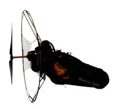
Designed more as an aid for finding thermals: The Mosquito E-Light from the German FTR. Motor HQ150 9 kW, full weight about 25 kg (of which 13 kg is the 37 Ah battery, battery life 20 minutes), full price with the charger and travel bag: 11000 €. https://www.moskito-light.com/moskito-e-light/
