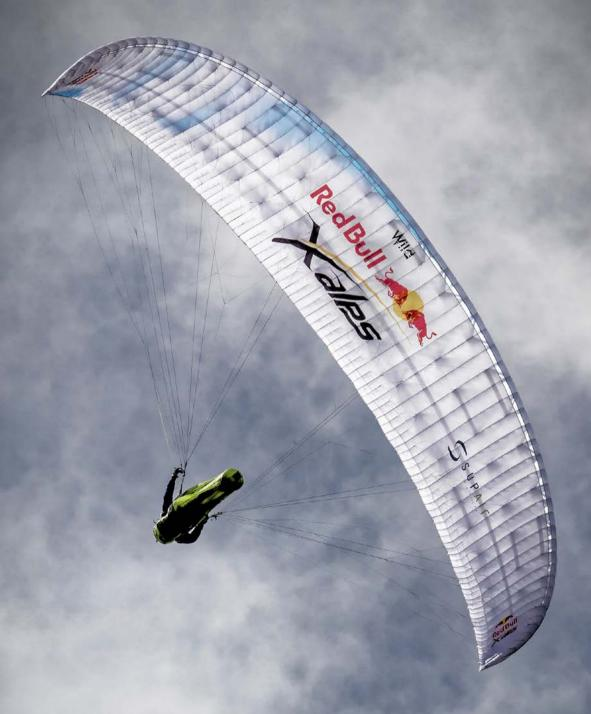
Benoit Outters on his Wild, which clearly reveals its internal structure in this beautiful photo by Niolas Assel. It's a three liner, derived from the Supair Taska, with a higher aspect ratio and an EN D instead of an EN C.
