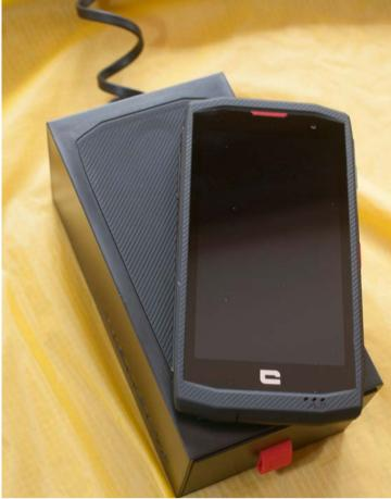
It isn't necessary to open the USB socket cover to charge the telephone: its box can be used as a cordless induction charger. It's just a bit longer.
