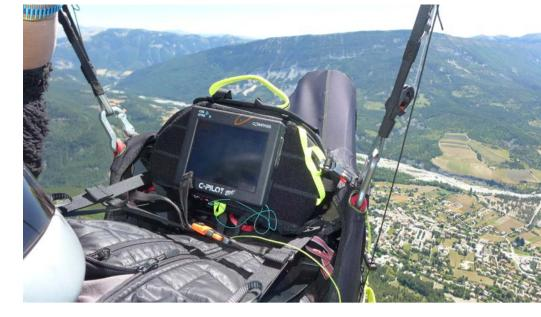
The upper part of the cockpit is removable so that you can take it to a briefing with the instruments attached. It has an integrated pocket for a USB battery.
