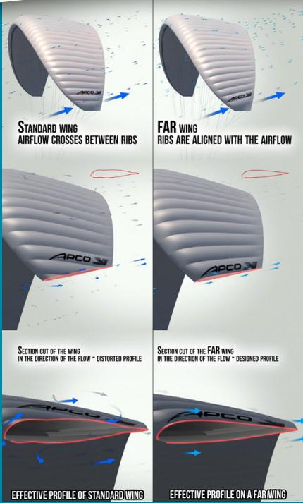
**Flow Aligned Ribs (FAR\*)** is a conceptual change in the way paragliders have been designed until today (Apco and the rest of the industry).
