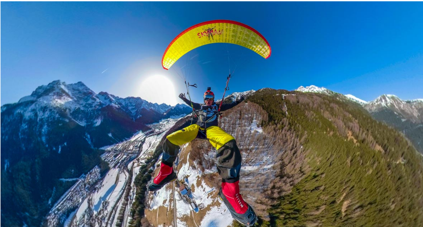
Markus Gründhammer on the latest prototype of the Hyper 7.01: 7.01 aspect ratio, 41 km/h hands up and about 53 km/h accelerated. Even at maximum speed, the wing behaves like a paraglider with normal performance, without any parasitic movement, according to Markus.
