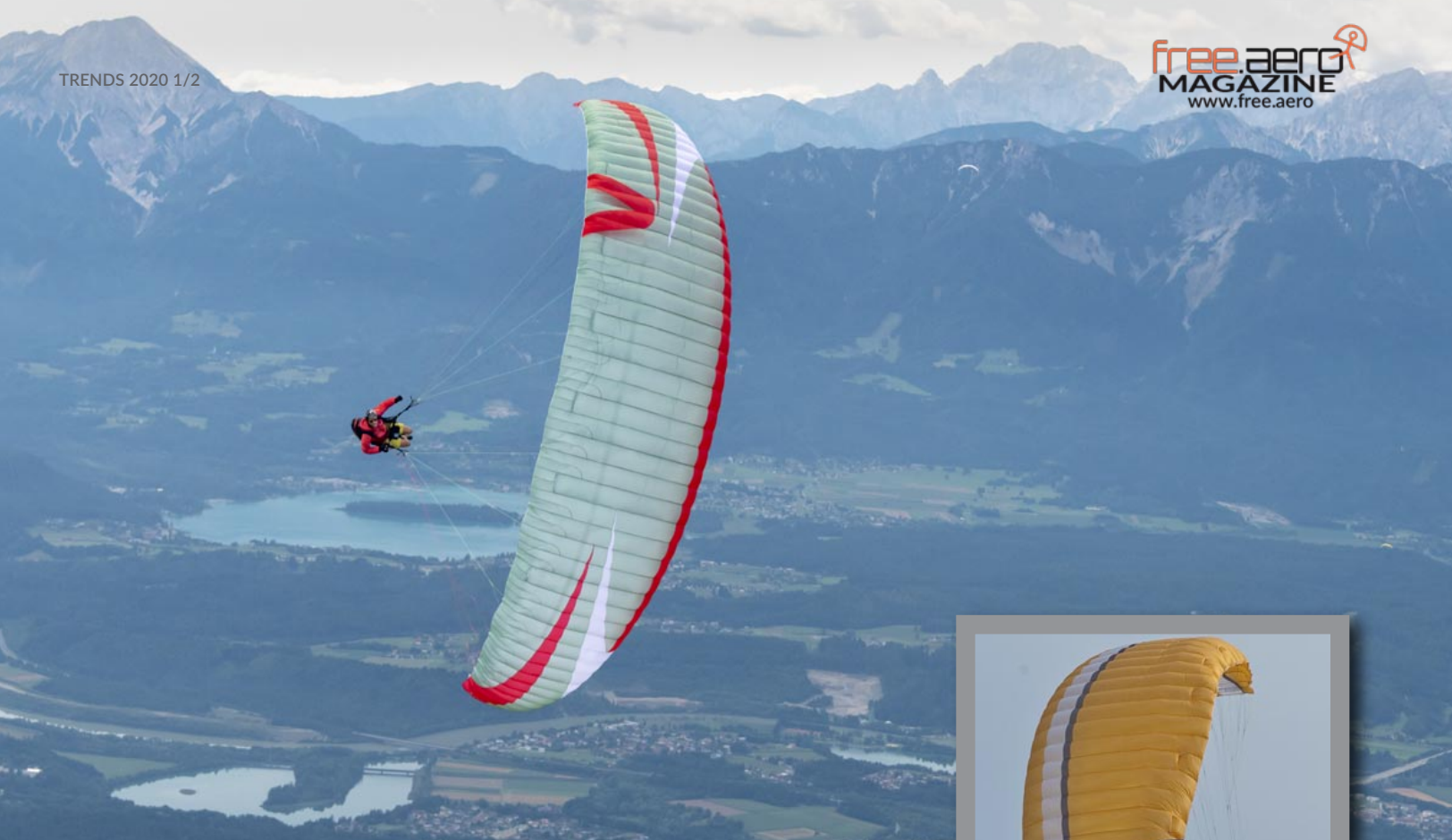
Skywalk Arriba 4: Jetflaps (the six slits in the trailing edge) and mini ribs with internal stitching (here in the form of a 'J') Photo: Skywalk
