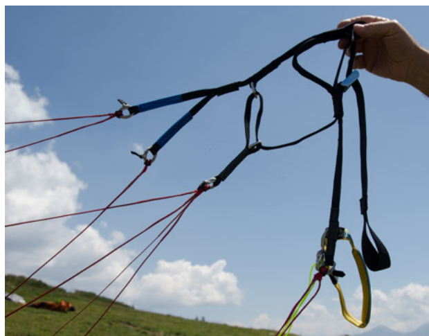
Strap risers. There is a Dyneema version with rudimentary trimmers, giving a further gain of 300g.
