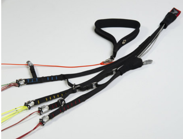
In accelerated flight, when flying using the rear risers, the Bs are also shortened.
