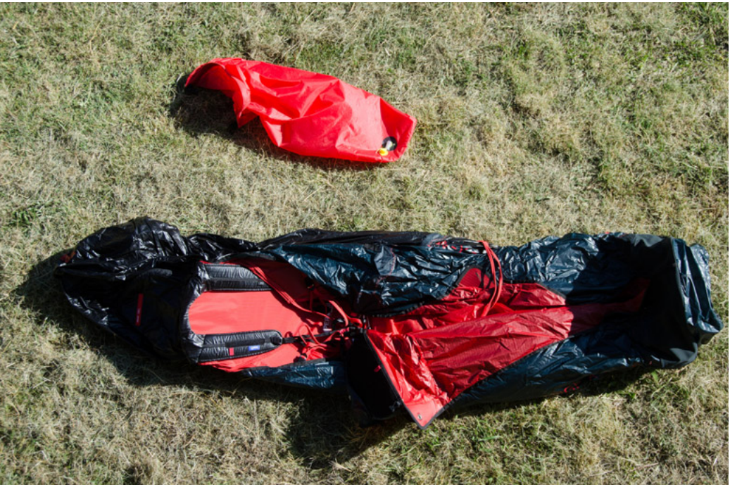
When we were unfolding it, we noticed the predominance of a fabric which resembles Skytex 32. But, in fact, it's a different fabric, Robic 32 g/m 2
