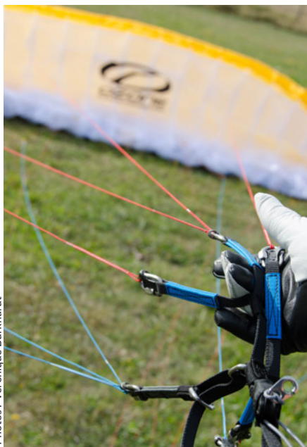
The risers are relatively simple and light.
