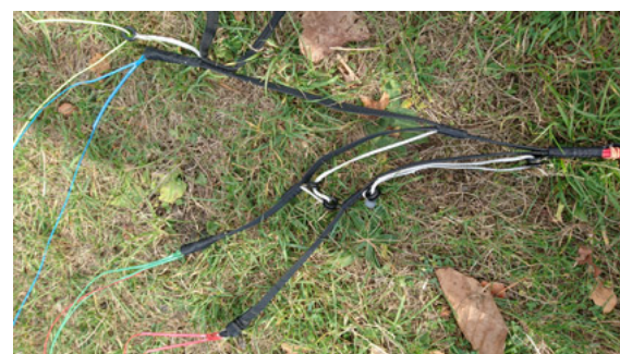
A wide riser, but without any metal. Even the hooks on the accelerator have been replaced by a ball.
