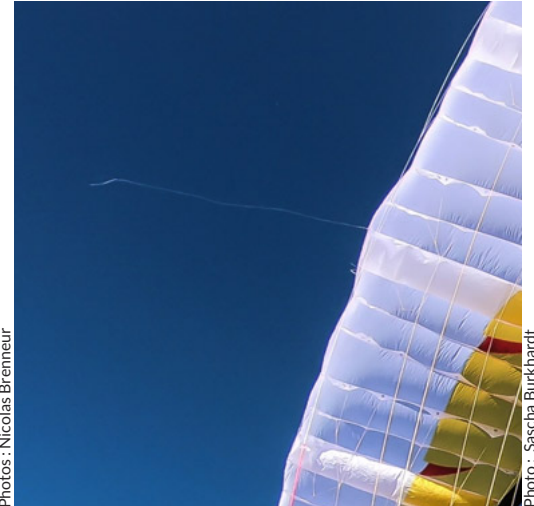
Not serious: unlike knots, this type of incident is totally benign, a thin brake line which breaks, shown here after a windy take off on rocky ground.
