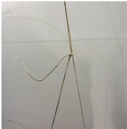
Not very serious: a case where a splice opens. The line, nevertheless, remained blocked in the right place.
