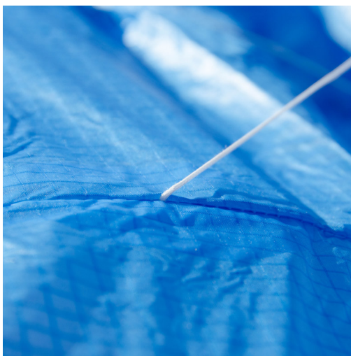
The lines are sewn inside the cells
