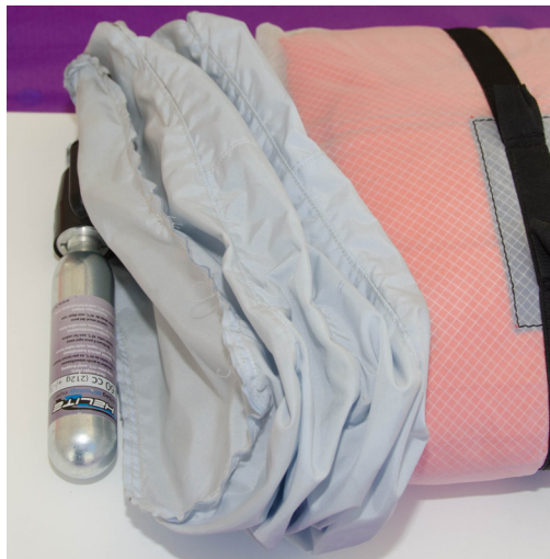
This 'airbag' fills with gas and ejects the reserve.
