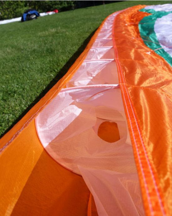
At GIN, the system to equalise pressure, in the same vein as the SharkNose, is called EPT,
