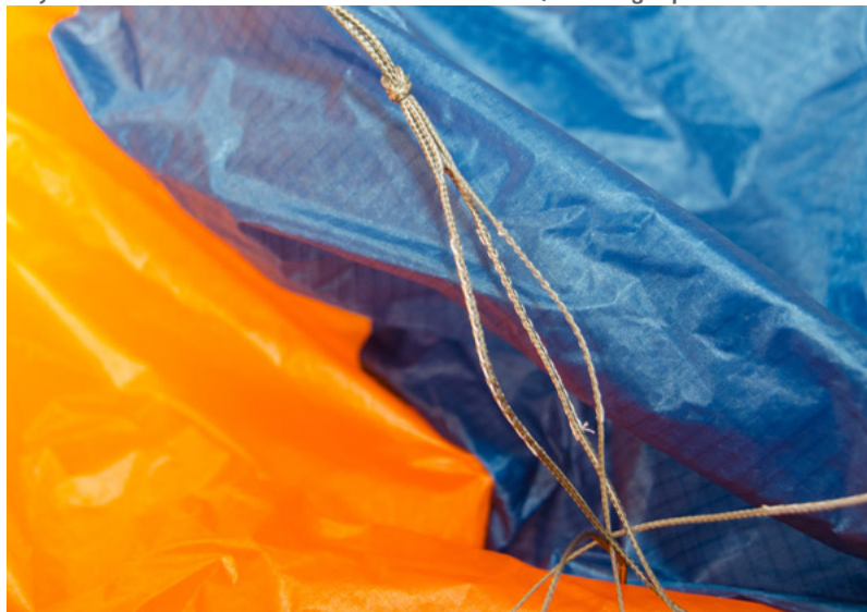
Very thin and unsheathed: the 0.5 mm Edelrid lines 8000/U-050 high up.
