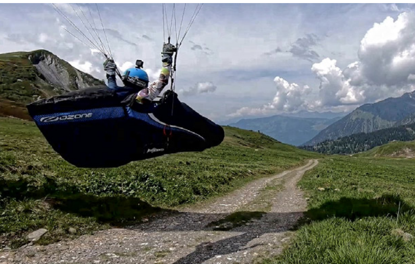
For distance flying, the fairing at the back of the Exocean has been optimised to improve performance. Photo: Philippe Goutagny
