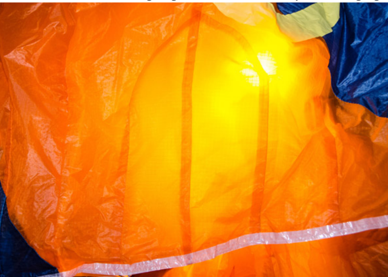
The stitching brings three-dimensional stability to the trailing edge.
