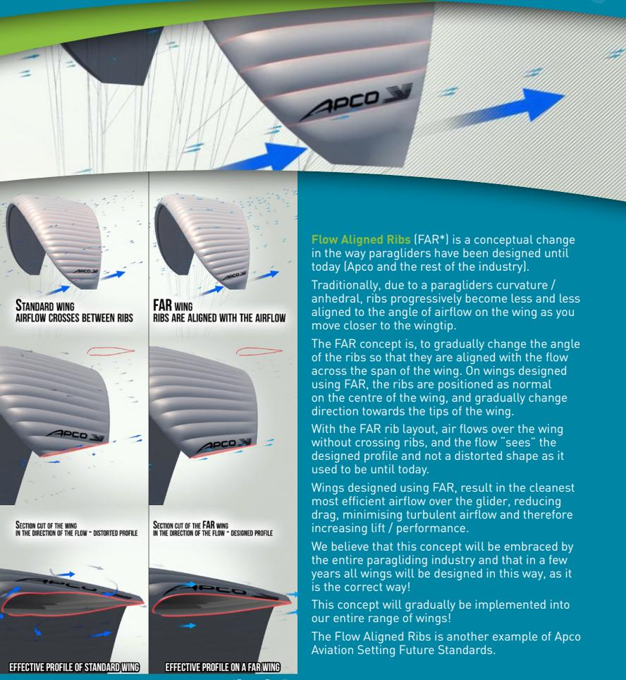
**Flow Aligned Ribs [FAR\*]** is a conceptual change in the way paragliders have been designed until today (Apco and the rest of the industry).
